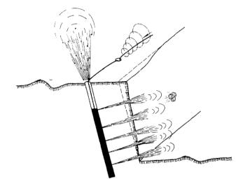
Fig. 1. Air blast fronts in blasting (Jimeno et al. 1995)
